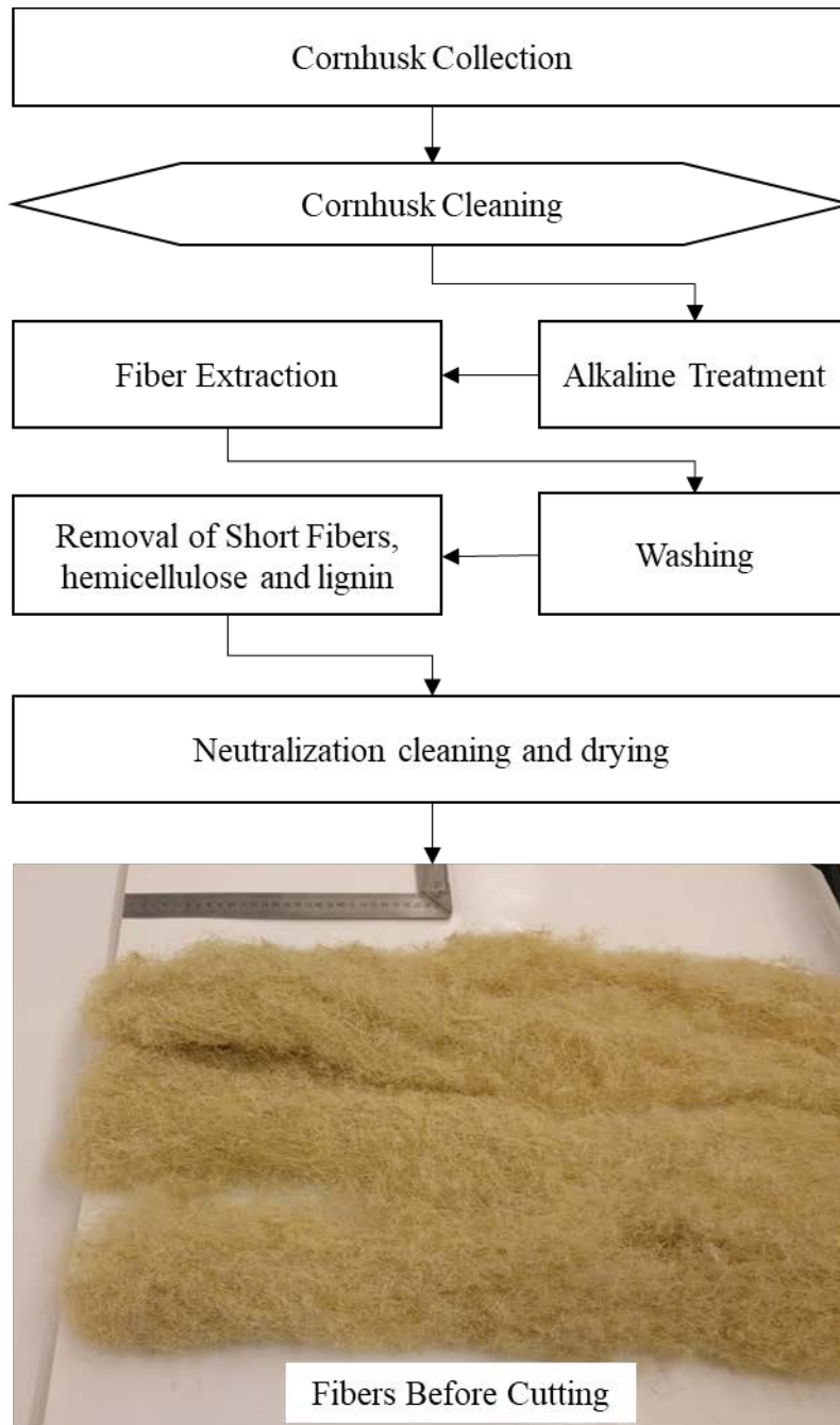
Figure 4: Cornhusk fibers fabrication scheme.
