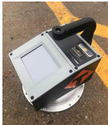
Figure 2. Pavement quality indicator (PQI).
