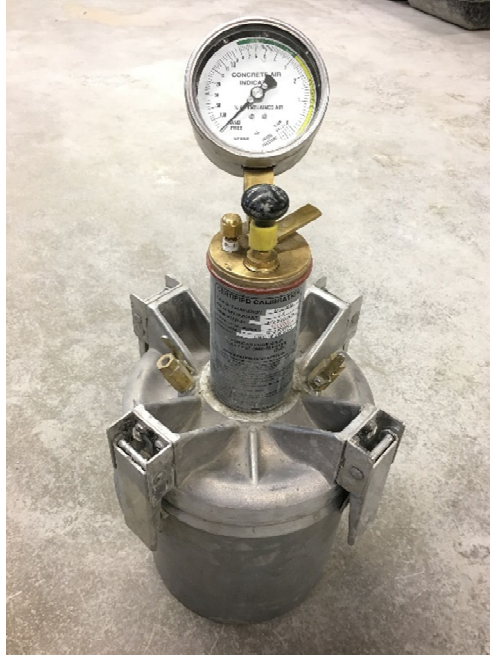
Figure 3.7. Air pressure meter
