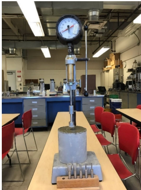
Figure 3.8. Setting time test setup
