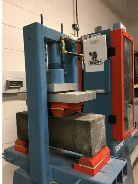
Figure 3.13. Flexural strength test setup
