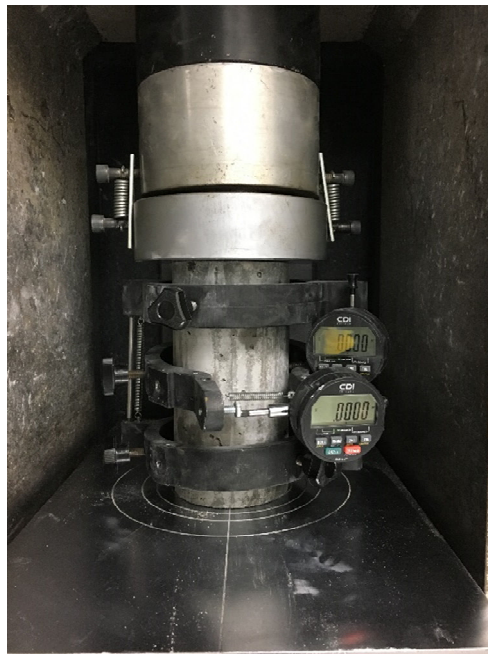
Figure 3.14. Static Modulus of Elasticity test setup
