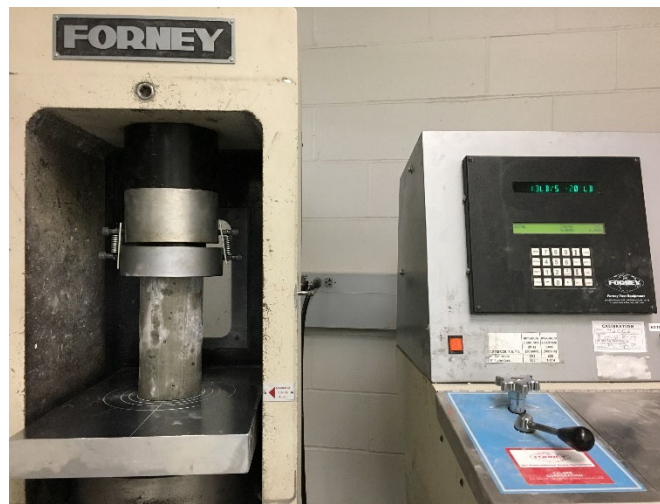
Figure 3.12. Compressive strength test setup
