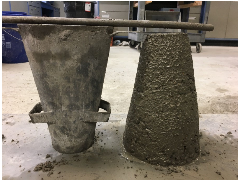
Figure 3.6. Slump test setup
