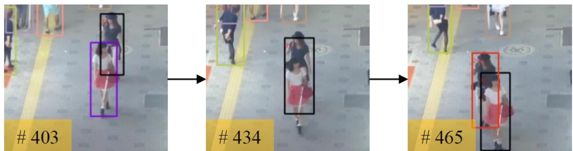
Figure 48: Identity switches to the other object that also appears in the same bounding box. Image from [20]
