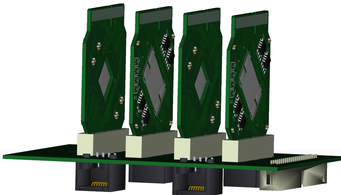
Figure 6.27: One of the two identical back-plane boards that make up the in-beam part of the telescope. The silicon micro-strip detectors are mounted at a 45 degree angle relative to the back-plane board, and each of the cards has board-edge connectors on both the top and bottom. This means that the cards can be rotated 180 degrees to change the relative orientation of the strips. They can be alternating horizontal-vertical (as shown), all vertical, all horizontal or any combination according to the operator's needs.
