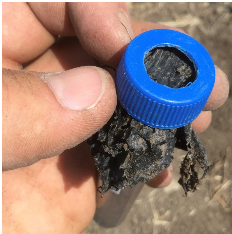
Figure 5: Conical tube and drilled cap apparatus to secure mulch fragment for piercing with force meter.
