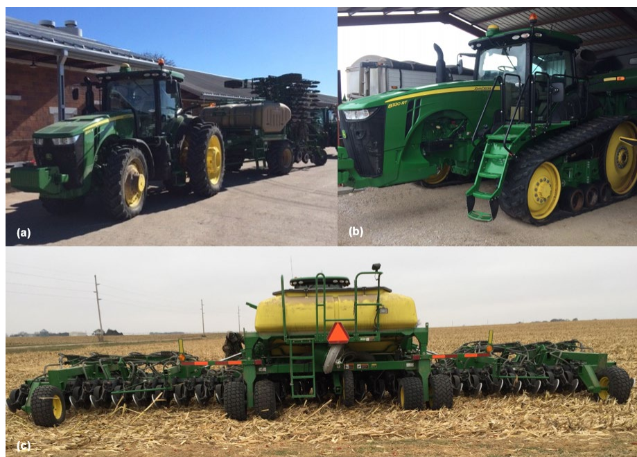
Figure 5.1: (a) JD 8320R with Great Plains NTA2007 no-till air drill used throughout wheat planting operation and (b) JD 8320RT and (c) JD 1990 no-till air drill used throughout rye planting operation.
