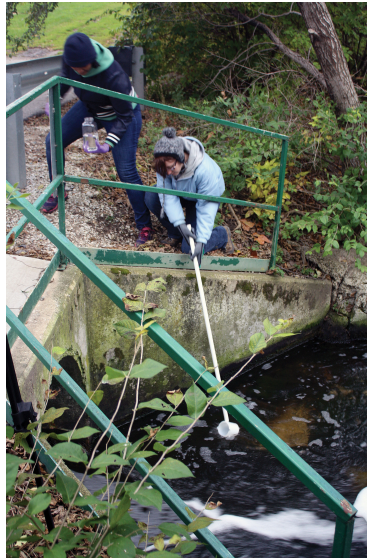
Collecting treated wastewater effluent from the Urbana WWTP
