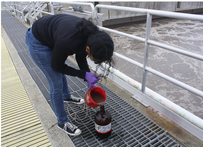
Collecting a wastewater sample from the aeration tanks at the Champaign WWTP.
