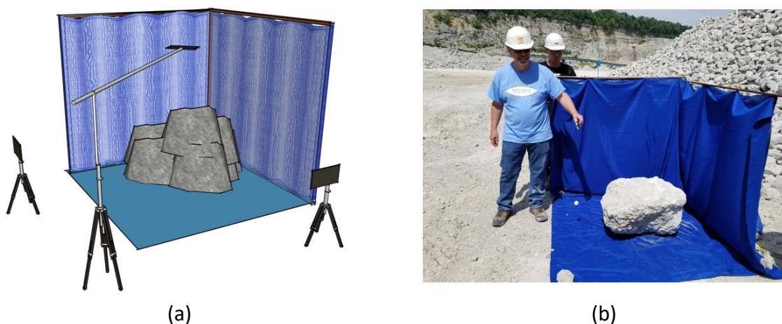
Figure 3.4. (a) A conceptual illustration and (b) the actual constructed setup of the field-imaging system for single rocks.
