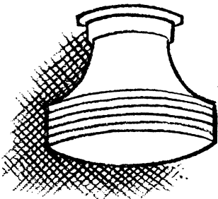
Fig. 19. Diameter of enclosing globe is 12 inches; 150-watt filament bulb.
