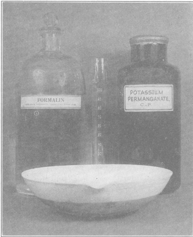
Apparatus used in making formaldehyde gas. The graduated cylinder is necessary for measuring the formalin. Pans should be of earthenware or porcelain.
