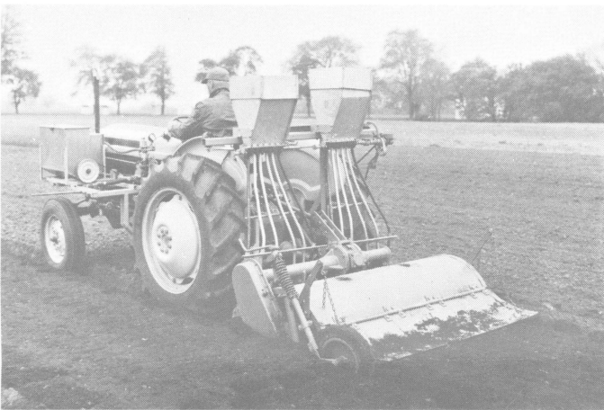
Figure 6 —Application of a granular nematocide at time of soil preparation. This method is especially suitable for preparing ground beds for cuttings to be grown for a year prior to transplanting to the field.
