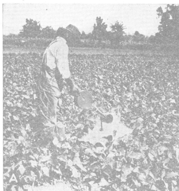
Fig. 4. — Small bellows duster suitable for home garden use. (U. S. Dept. Agr.)
