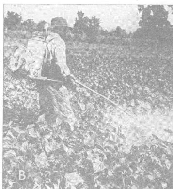
Fig. 5.—Knapsack bellows type of duster for truck garden and small field use. (U. S. Dept. Agr.)
