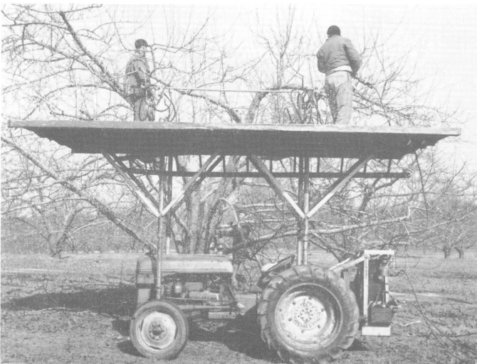
Fig. 3.—Some growers have built platforms similar to this one in order to help make the use of power pruning equipment more efficient.
