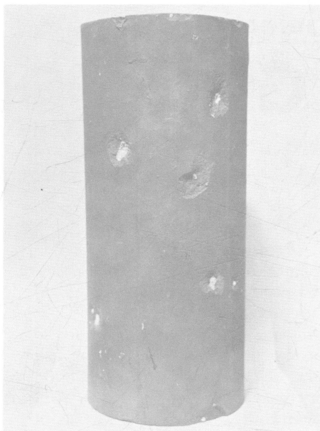
Clay tile with flaking caused by lime spots and pebbles.
