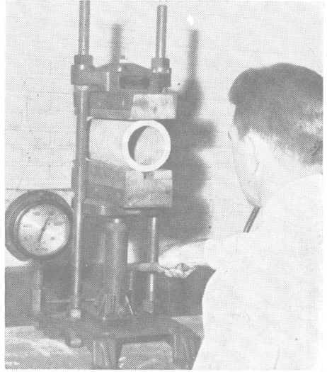
Tile being tested for strength in hydraulic press.
