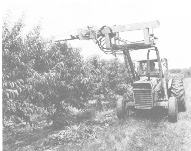
Fig. 32: A hydraulically driven sickle blade mower can be mounted on a forklift and used to top hedge peach trees during summer.
