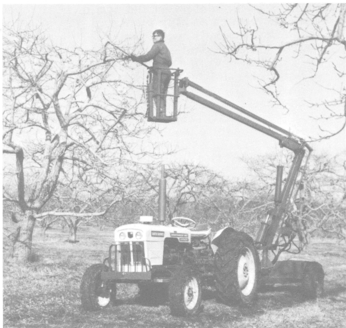
Fig. 31: Hydraulically controlled towers and pruning equipment increase worker efficiency. This equipment operates from the tractor hydraulic system.
