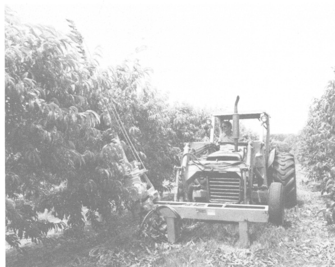
Fig. 33: Peach tree size can be maintained in high density plantings with a sickle blade mower mounted on a forklift.
