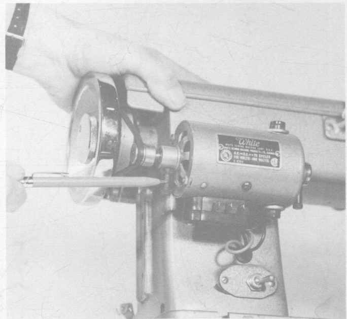
FIGURE 6. Lubricate motors that require oiling or greasing, once a year.
