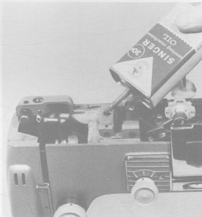
FIGURE 2. Put one drop of oil in each oil hole every 5 to 10 hours of use.
