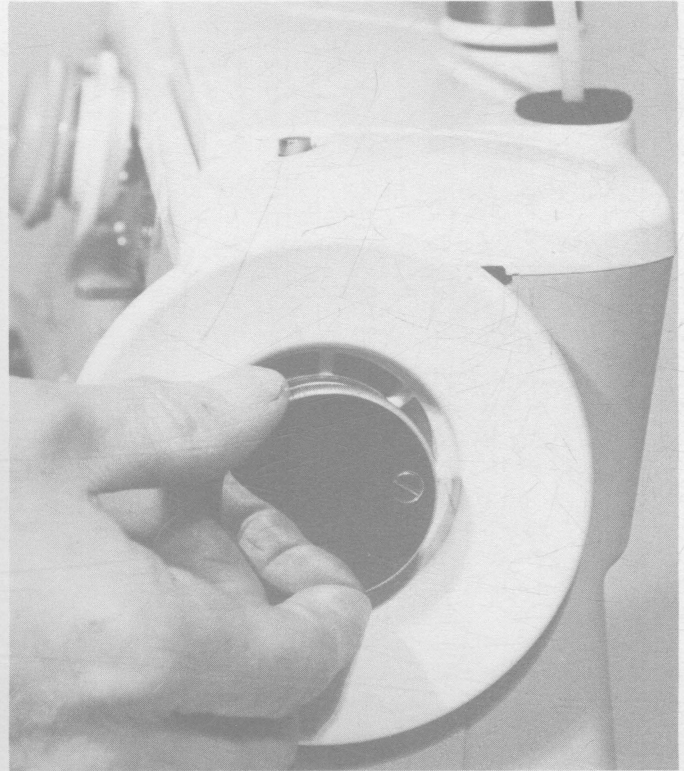
FIGURE 5. Do not oil or grease the hand release clutch or it may slip, and the machine may not sew.
