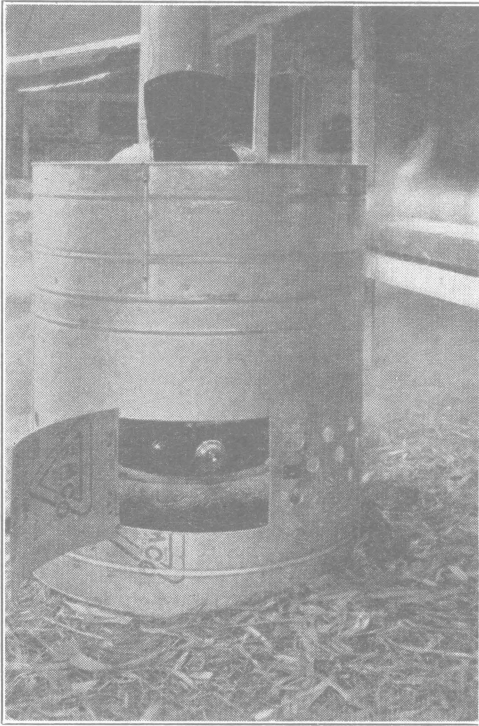
Fig. 8.—An ordinary heating stove with a metal jacket around it proves very satisfactory.
