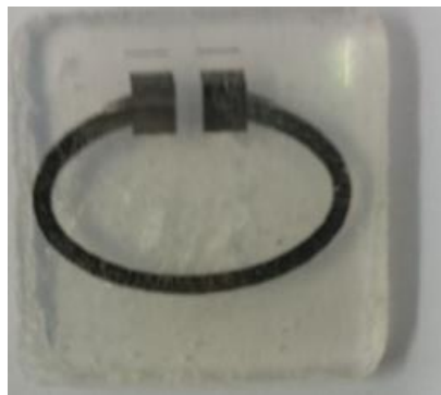
Fig. 2. Inkjet Printed Conductive Loop on PDMS Block
