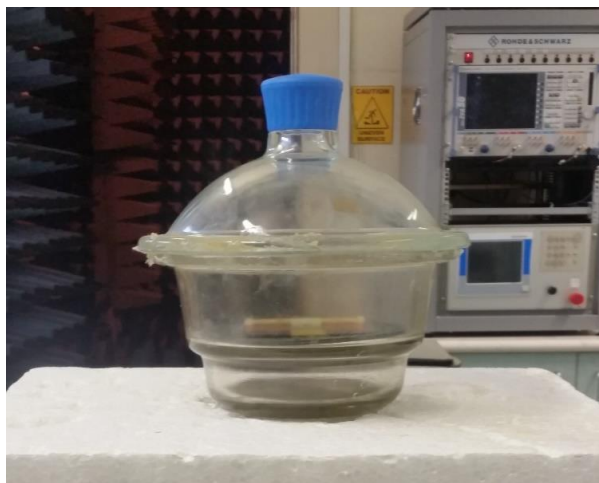
Fig. 3. RFID Tag with PDMS loop inside desiccator during measurements
