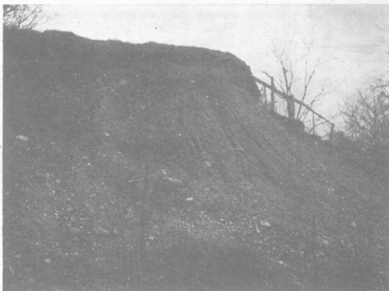
"Drift soils are distinguished by the presence of rounded boulders." Notice the line of true soil at the top of the bank.
