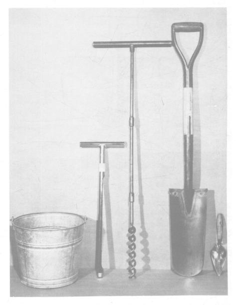
A clean bucket, spade and knife, a soil probe or an auger. A soil probe or an auger is best because it helps to secure equal amounts of soil to a definite depth at the sampling sites.
