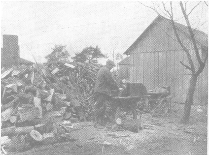
Figure 17.—Mr. J. C. Rausch says that with his 5-hp. portable motor, he was able to "buzz" as much wood per hour as he did formerly with a tractor for power.
