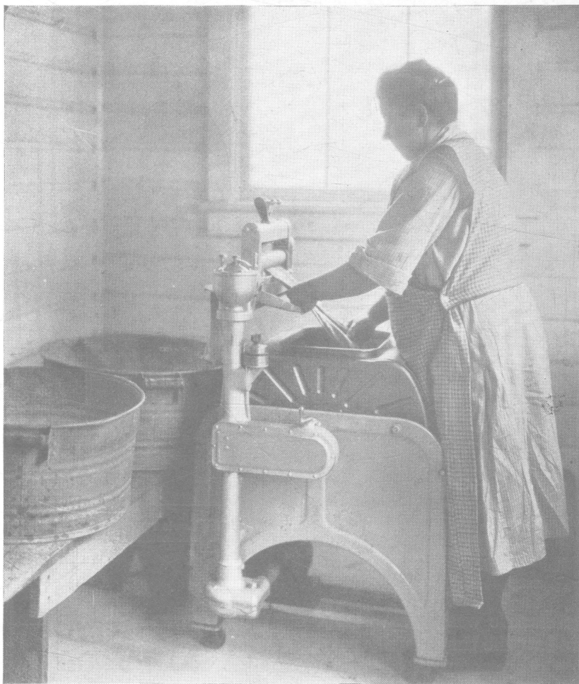
Figure 5.—The electric washer saves time and energy. Two kw-hr. of current operates Mrs. Charles Nicol's washing machine for one month.
