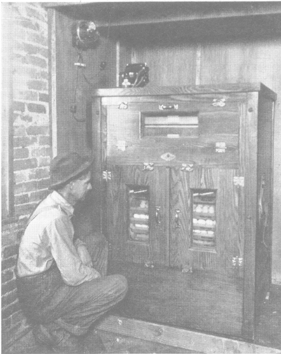
Figure 19.—Mr. Peter Renner is well pleased with the operation of his electric incubator. This is a 1000-egg size, and uses from 7 to 8 kw-hr. per day.
