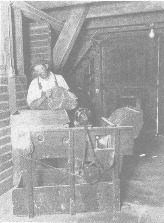
Figure 18.—A small motor ( \frac{1}{4} hp.) takes the place of one man on such jobs as this. One kw-hr. of electricity will operate this size motor for 4 or 5 hours to run fanning mills, emery wheels, grindstones, and other small machines that may be turned by hand or driven by a small electric motor.
