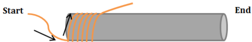
Figure 7: Diagram of beginning winding of the coil around a core. Coil wound counterclockwise when looking down the core from the start.
