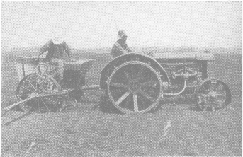
Fig. 13.—A two-row potato planter used for planting potatoes on muck. Potatoes are often profitably used in the rotation with onions.
