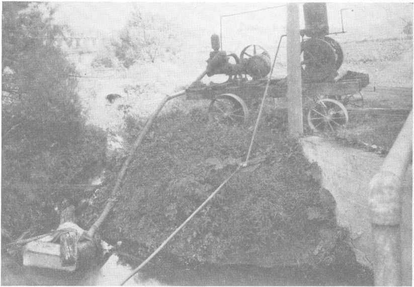
Fig. 11.—A portable pumping plant which supplies water for irrigating crops grown on the muck in the background.
