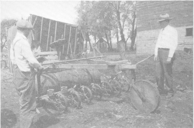
Fig. 4.—Multiple row seed drills are frequently used to plant onions on muck in Ohio. Note the handle on the left used to guide the drills.
