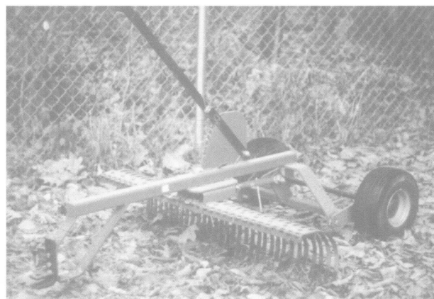
Figure 13. Weed control is needed for open sand bioreactors. In addition to grass and weeds, algae can grow on an open bioreactor surface. Regular raking helps to prevent clogging. (Top) Raked and unraked sand bioreactors. (Bottom) Rake for maintaining sand bioreactor.
