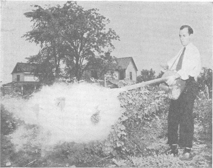
The fan-type duster, driven by a crank, gives an even flow of dust. It is effective for use on currant worm and dusting backyard plants and trees.
