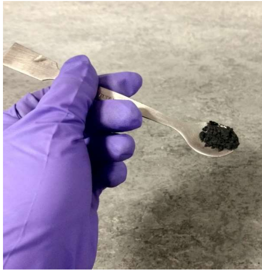
Figure 4.18: Aspect of the milled carbon fibre (Carbiso™ MF) used for the preparation of composites
