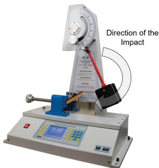
Figure 6.8: Representation of the Charpy impact test.
