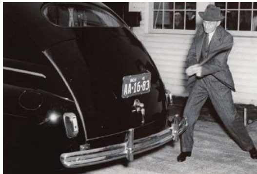
Figure 3.3: Henry Ford demonstrating the performance of an external body part produced with hemp fibres. 19
