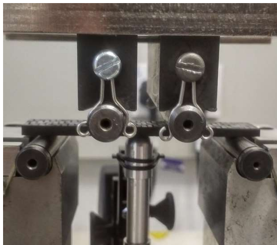
Figure 7.12: Illustration of the four-point bending flexural test.
