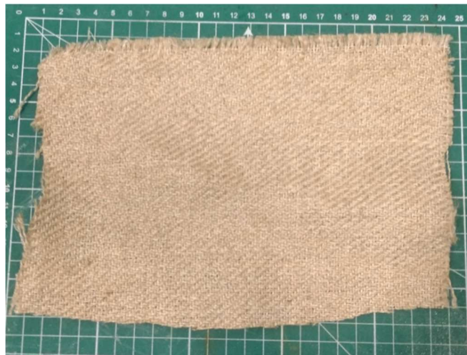
Figure 6.1: Representation of the woven flax fibre mat utilised as reinforcement for the manufacture of biocomposites.
