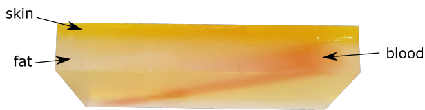
Fig. 5: Gelatine phantom comprising skin (yellow), fat (white) and blood vessel (red)
