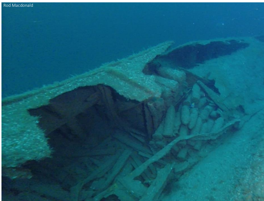
Figure 102: A view from forward, looking aft of the port 6-inch shell room showing separation and collapse of hull bottom (right) from port side of the ship (left)
