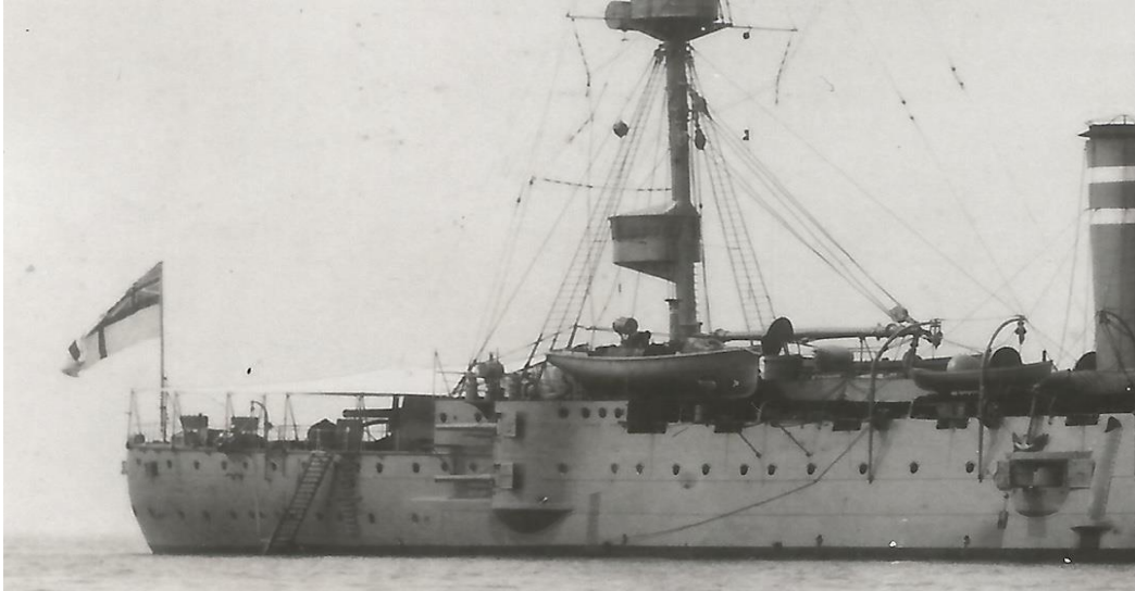
Figure 8: Aft view of HMS HAMPSHIRE showing twin superfiring casemate just abaft the main mast
