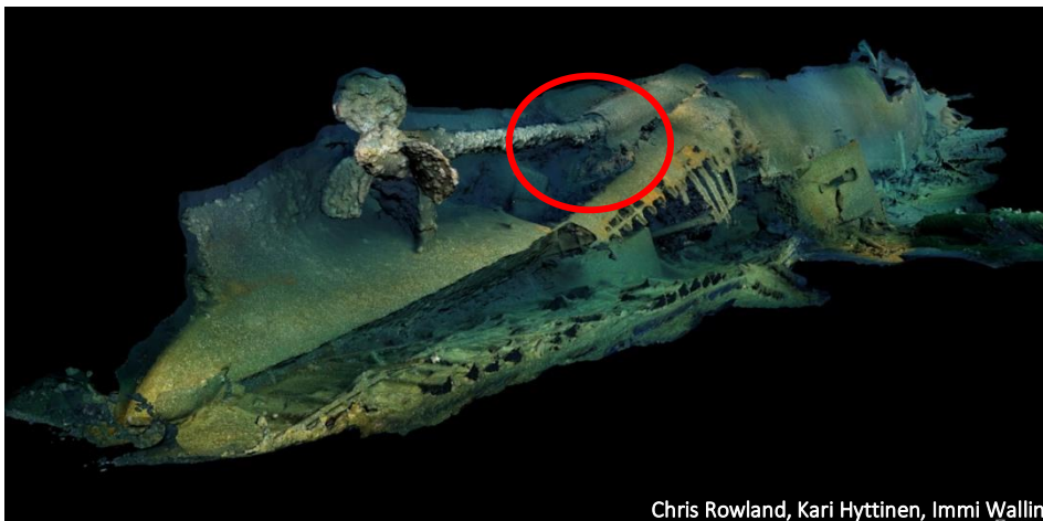
Figure 134: 3 image of port side propeller and shaft
