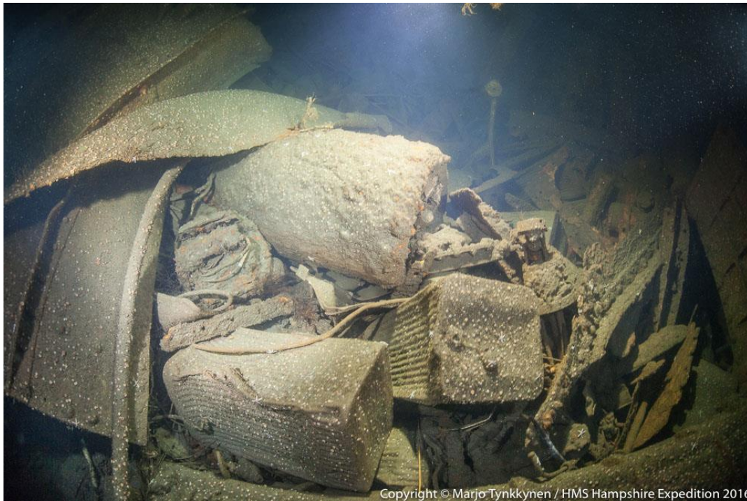
Figure 54: 7.5-inch flash-proof ribbed brass cordite storage boxes in vicinity of P & Q-turret magazine
