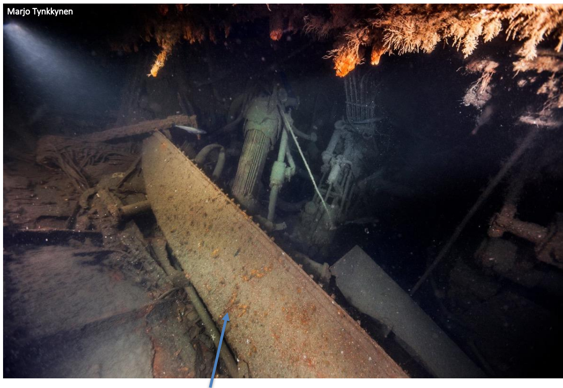
Figure 79: The aft end of the port bilge keel is visible in the fissure lying alongside evaporators
