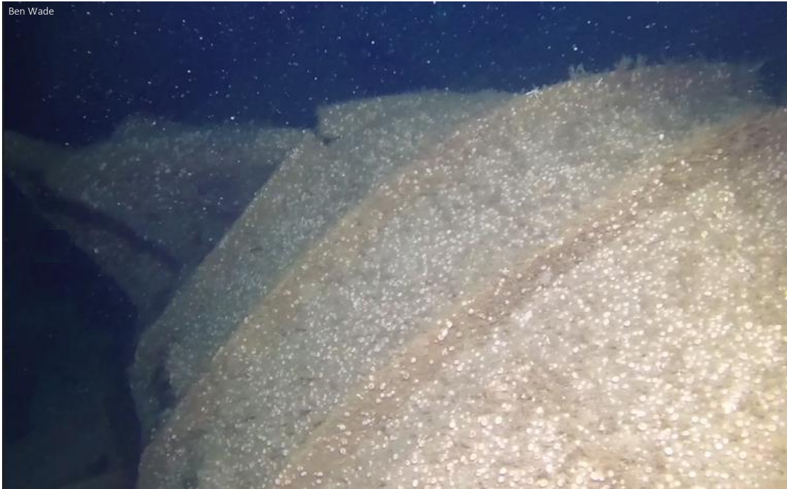
Figure 121: Bulkhead looking to port across the ship: note the cracking damage
