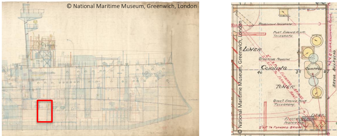
Figure 57: Plans of Lower Conning Tower
