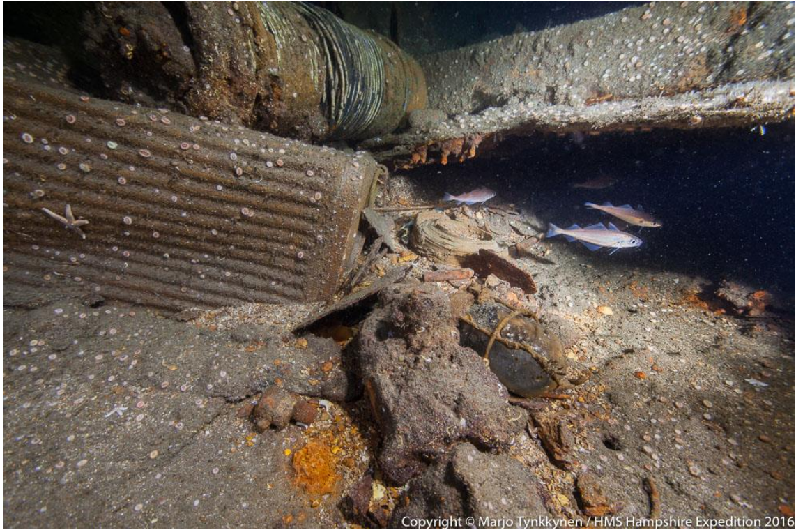
Figure 104: A brass cordite case. A cage lamp with glass intact lies to its right
