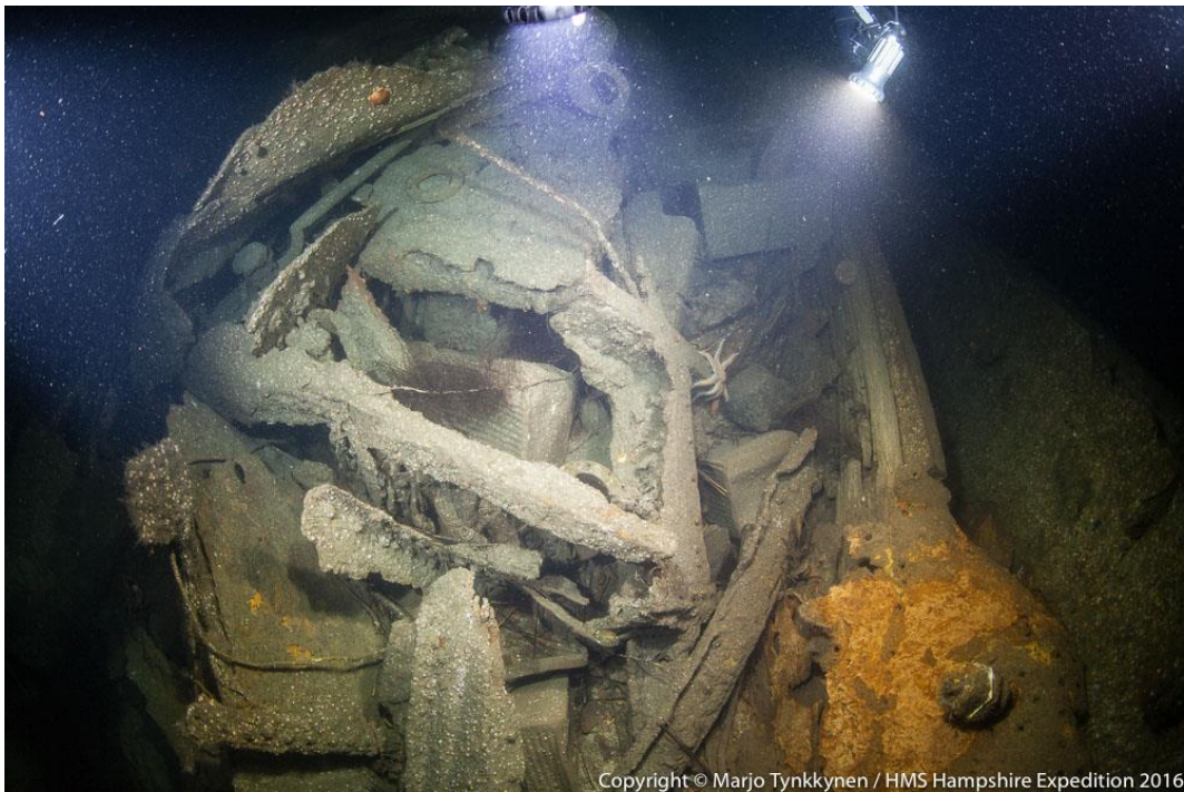
Figure 53: Cordite in ribbed brass flash-proof storage boxes lie in the bow wreckage adjacent to internal timber support for the armoured belt. Note the large stud nut in bottom right
