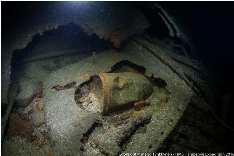
Figure 56: A brass torpedo warhead casing showing hydrostatic pressure damage (The degree of damage suggests the warhead is not loaded with explosive and might be for drill or practice)
