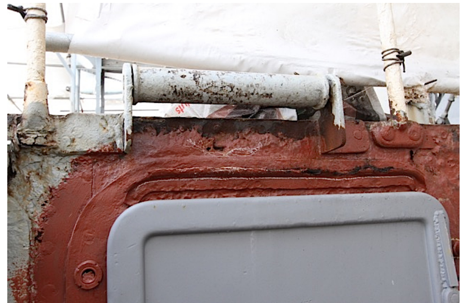
Fig.15: Poorly fitted watertight door
