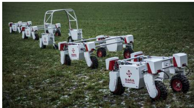
Fig. 3: Various robots made from Thorvald II modules
