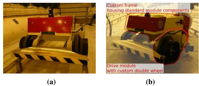
Fig. 4: The presented robot is designed for use in a greenhouse environment. (a) The robot on rails; (b) the robot on the headland floor. One of the two drive modules and the custom sheet metal frame has been highlighted.
