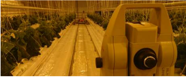
Fig. 10: Ground truth poses are obtained using a total station
