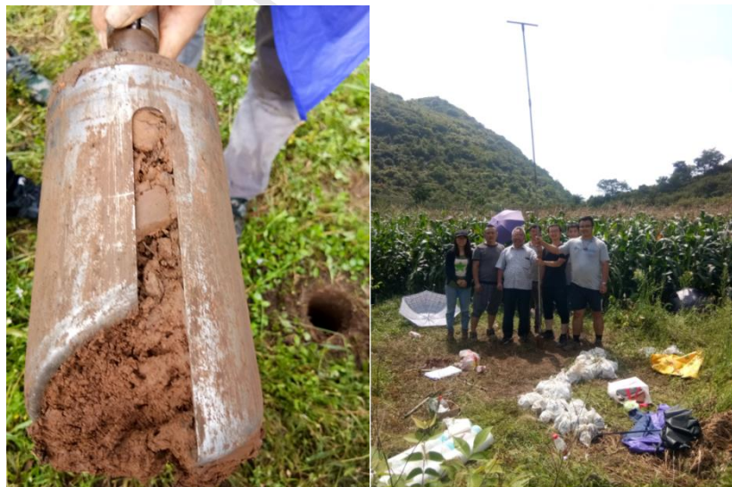
Fig.5 Auger soil for depth verification
