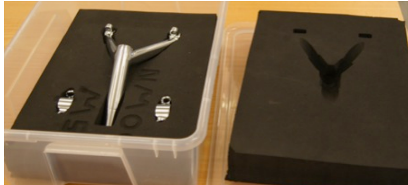
Figure 8. Finished example packaging manufactured from neoprene foam
