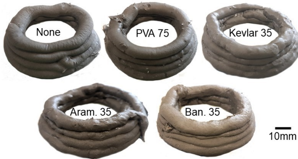
Figure 4. Buildability tests with four fresh circular layers extruded by the powered deposition device for each mix shown.
