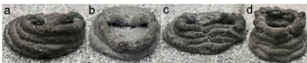
Figure 4. Buildability tests with circular layers extruded from the syringe device, (a) control mix (b) PP1.2 (c) ARG1.2 and (d) PVA1.2. PVA fibres provided the most buildable mixes.
