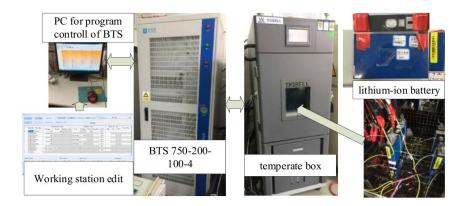
Fig. 3 The experimental platform
