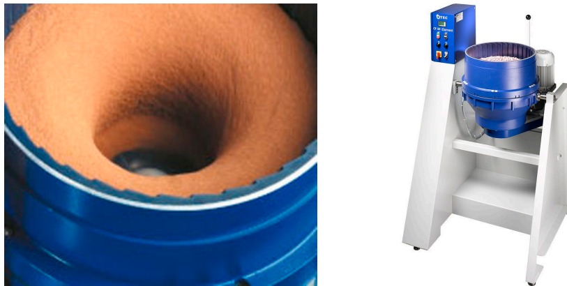
Figure 1. Centrifugal disc machine principle (LJMU).
