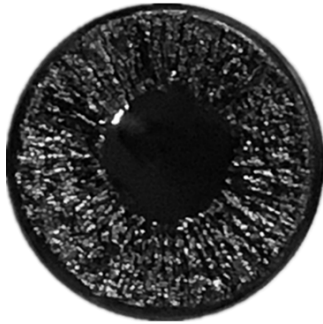
(a) A ‘factory roof’ morphology of cracking surface
