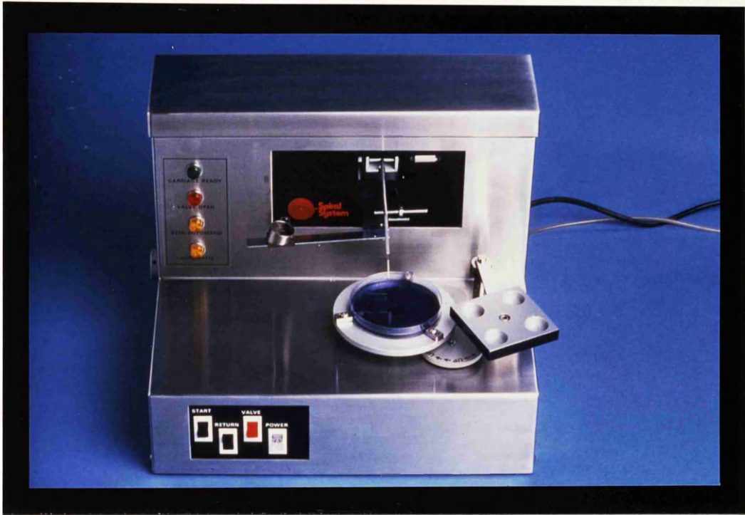
Fig. 2.14. Spiral plater in use with MSB plate in position.
