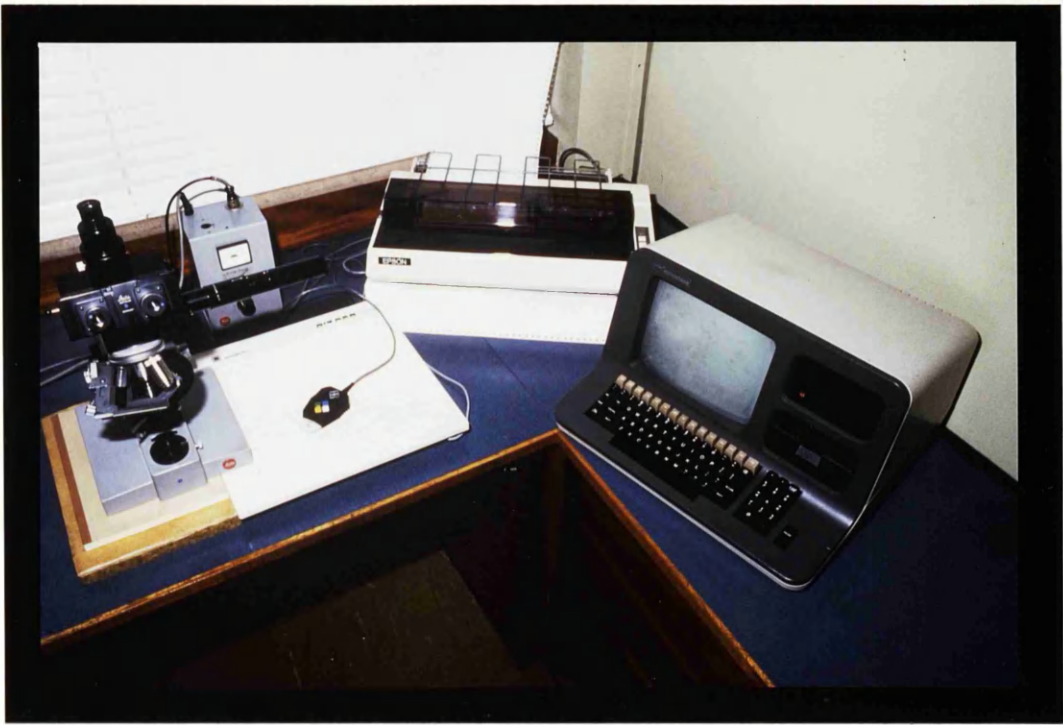
Fig. 2.8. Computerised planimetry equipment used for measurement of surface area of enamel slab.
