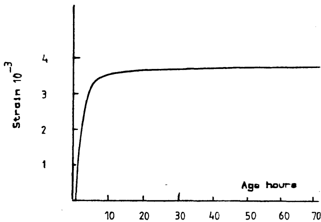
Fig. (1.33-a) Development of hardening shrinkage strain of resin concrete.
