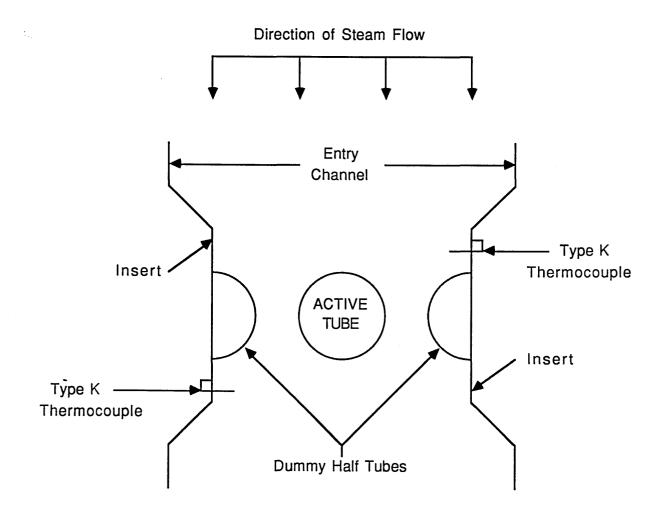
Figure 7:Side View of the Condenser Test Cell
