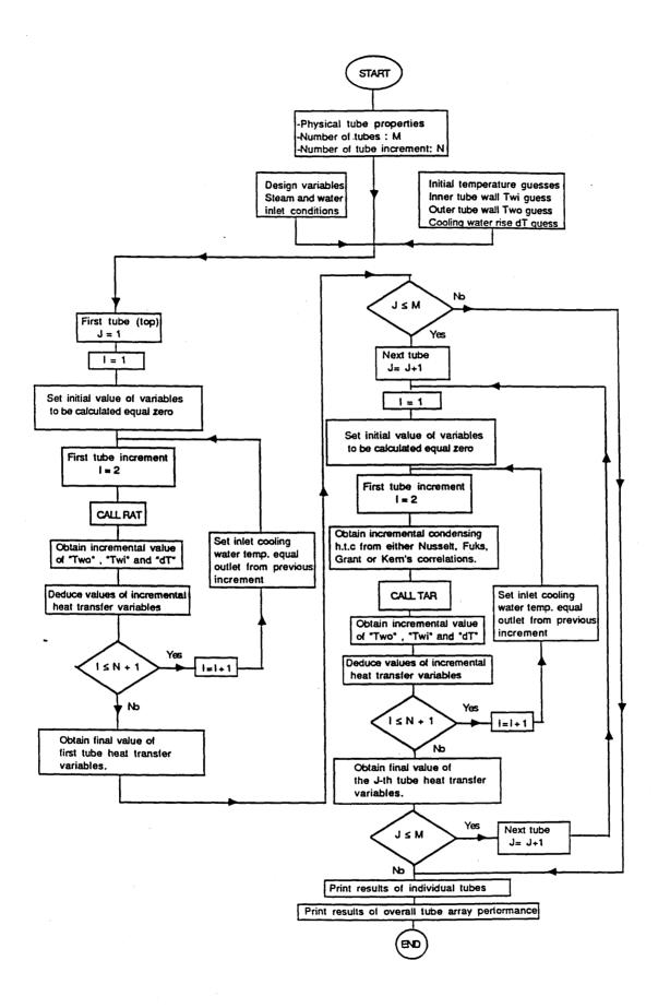
Figure 8: Flow Diagram of the Plain Tube Computer Program
