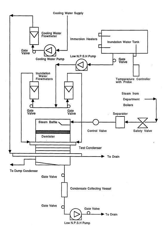
Figure 20:Schematic Diagram of the Experimental Apparatus
