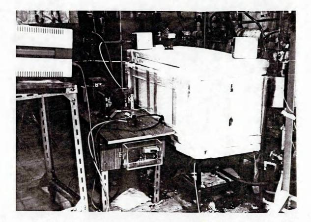
Figure 24:insulated Condensate Water Tank
