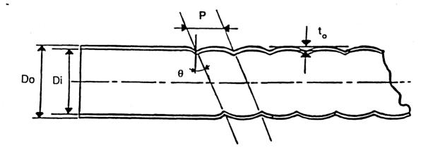
Figure 4: Typical Roped Tube Configuration with the Various Characteristics
