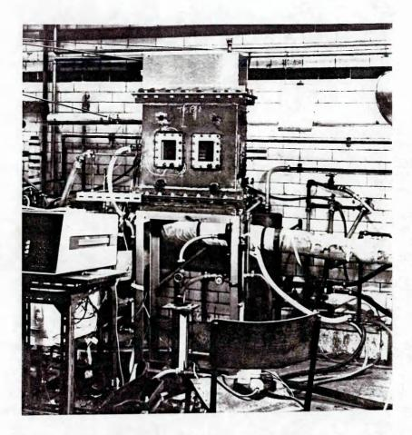
Figure 10: The Assembled Test Condenser Rig
