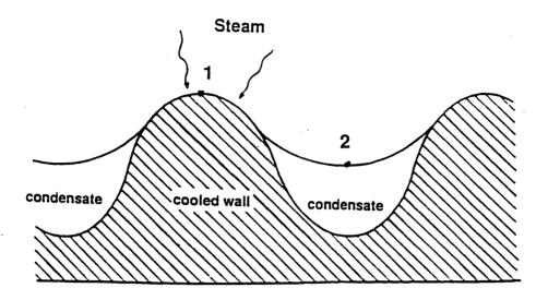
Figure 3: Cross Sectional View of the Profile of a Roped Tube
