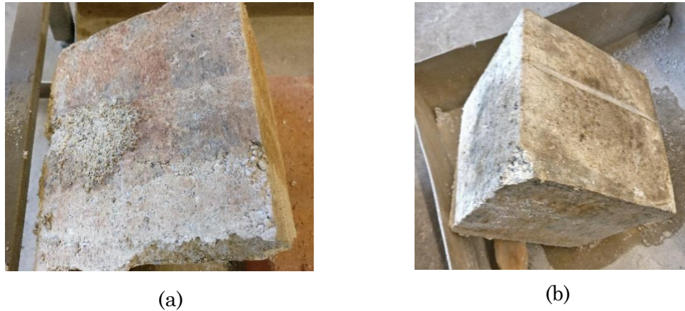
Figure 3.23. Eroded surface after durability tests (a) guar gum and (b) xanthan gum
