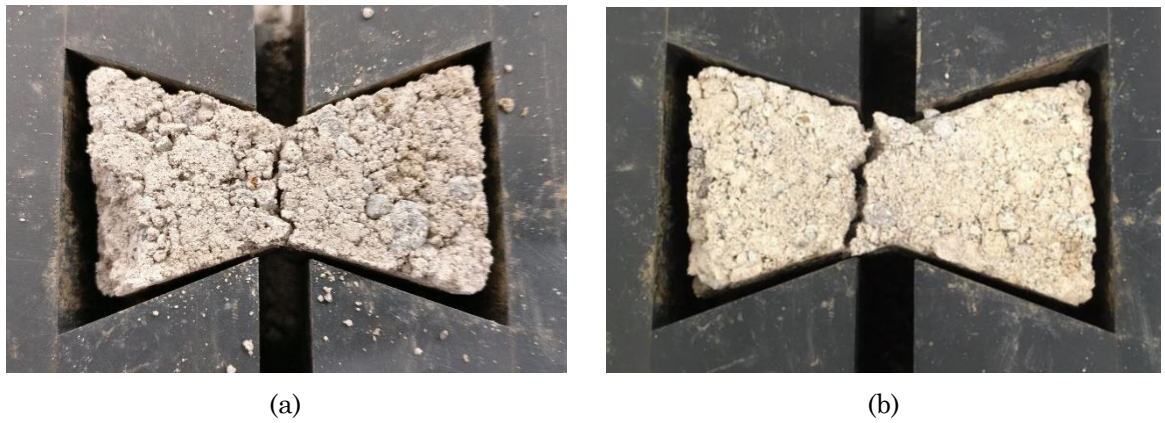
Figure 3.14. Failure patterns for 28-day tensile specimens for a) guar gum (b) xanthan gum
