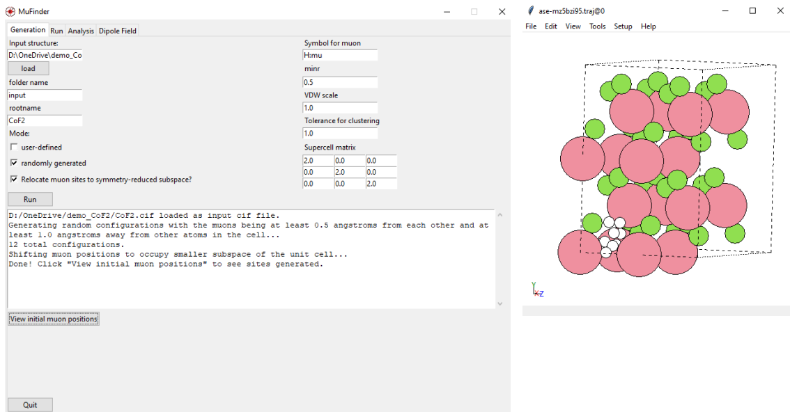
Figure 4.2: A screenshot of the MuFinder program, demonstrating initial muon position generation. Left: the main GUI window. Right: initial muon positions in a 2 \times 2 \times 2 supercell of \text{CoF}_2 visualised using ase-gui.
