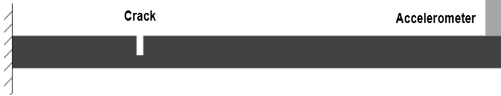
Figure 5: Schematic of cantilever beam with end mass
