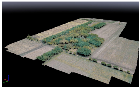
Figure 4: The 3D point cloud obtained from the RGB images
