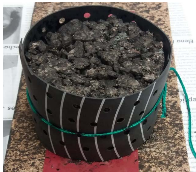
75 76 Figure 2. Marshall sample of cold porous asphalt before being dried by induction heating
