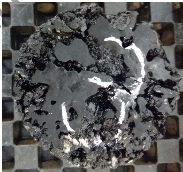
80 81 Figure 3. Bottom of a Marshall simple presenting a drainage problem after heating by induction
