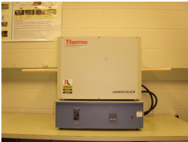
Figure 2.4 Thermal furnace for heating the O3-NCNFM precursor pellet
