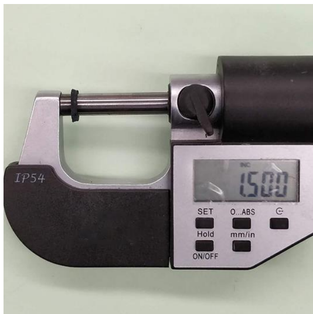
Figure S3.9 Measurement of the thickness of 8-layers patterned electrode
