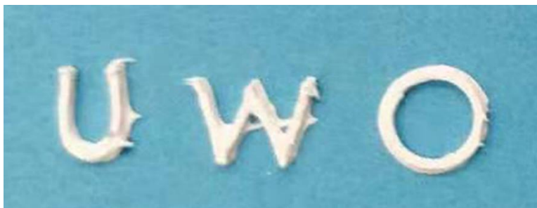
Figure S5.3 3D-printed LAGP with unique “UWO” letters before annealing
