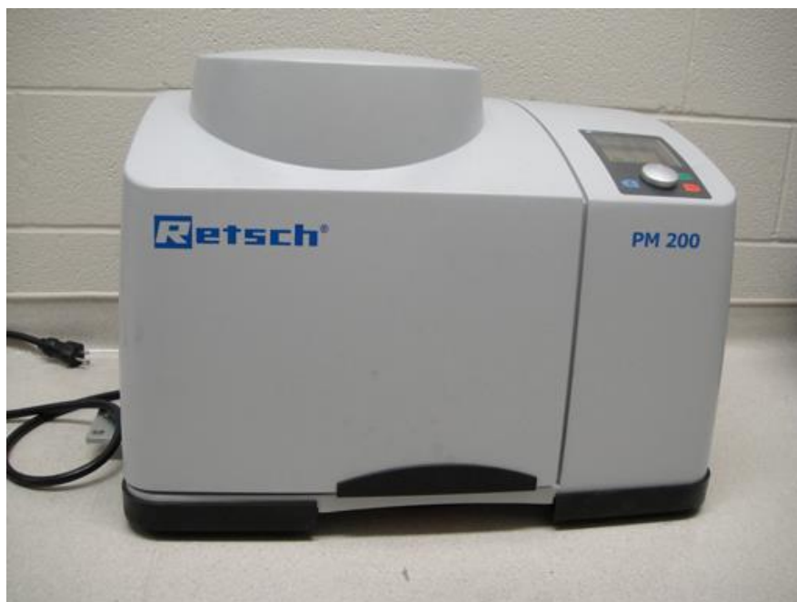
Figure 2.5 Ball-milling machine used for preparing P2-Na 2/3 Ni 1/3 Mn 2/3 O 2 precursor
