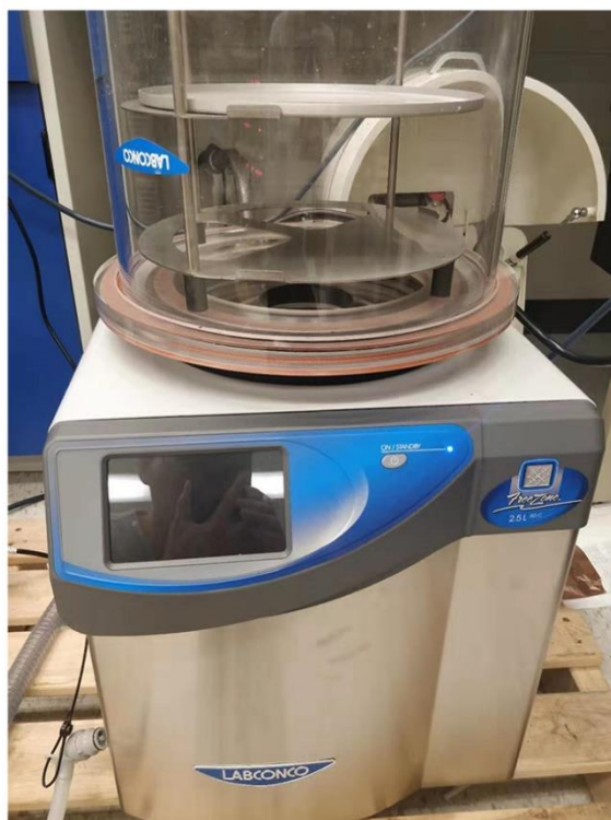
Figure 2.3 Freeze-Drier for drying the printed structures
