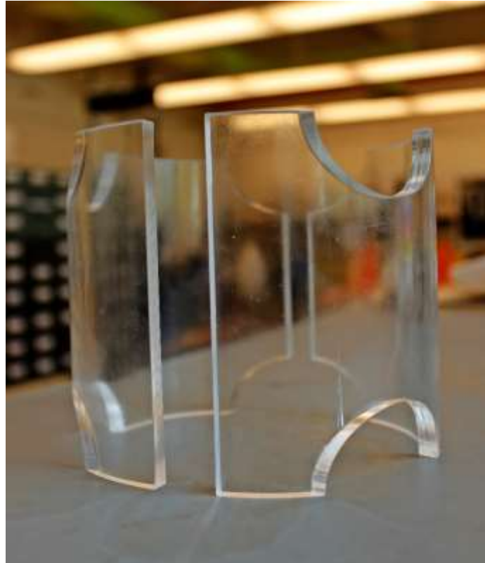
Figure 3.8: Image showing the acrylic spacers used to initiate K_0 consolidation
