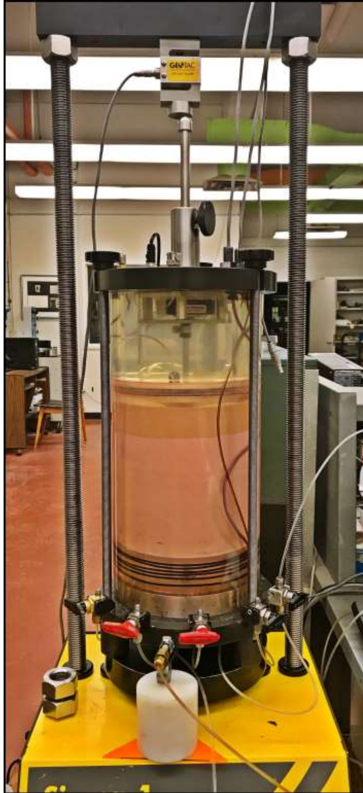
Figure 3.11: Fully set-up MCPT chamber during a test
