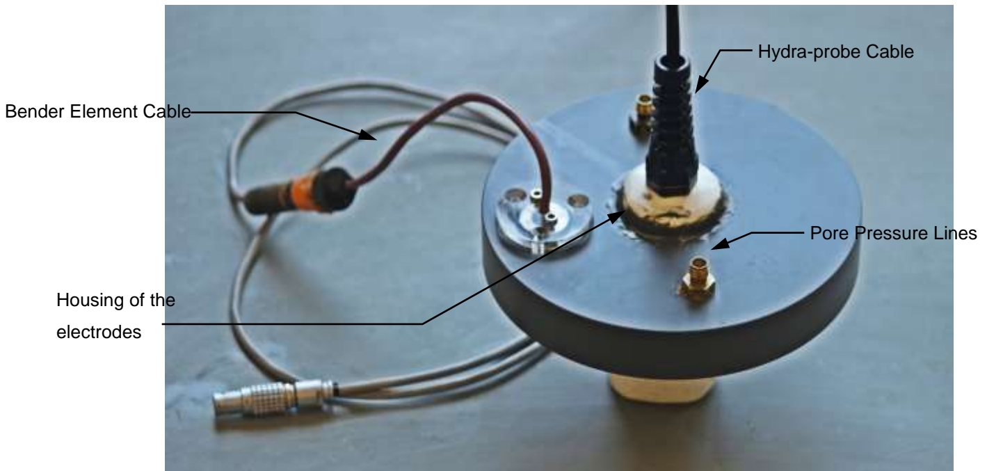
Figure 4.2: Illustration of the electrode cable on the upper side of the top cap
