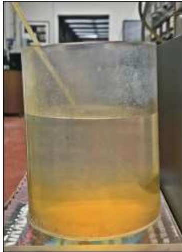
Figure 4.26: Presence of iron in outcoming water from a typical silica sand specimen
