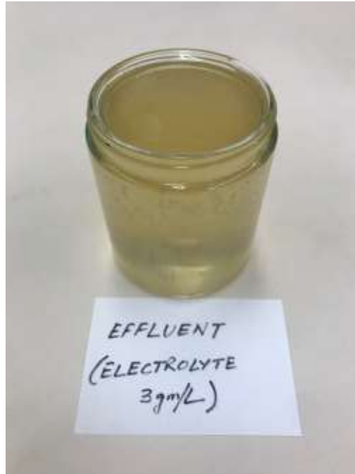
Figure 4.14: Image showing the effluent water after soaking Boler sand
