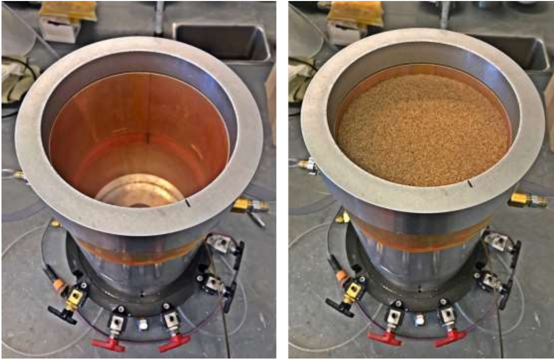
Figure 3.17: Assembled split mold before (left) and after (right) specimen preparation
