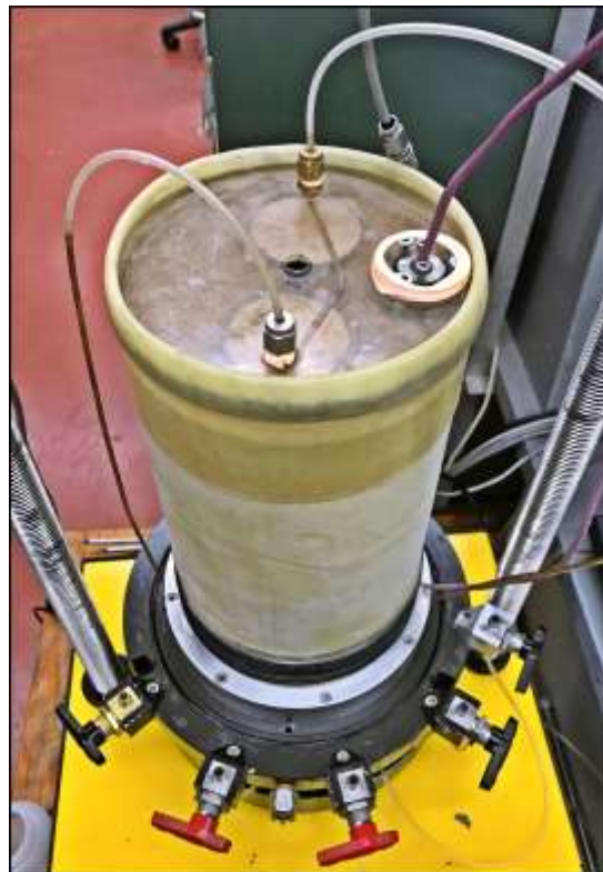
Figure 3.10: Central hole for cone penetrometer on the top cap
