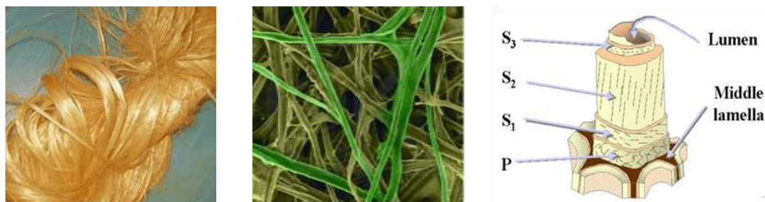
Jute Fiber structure Cellulose Fibers from Print Paper (SEM x1080) Jute fibre
