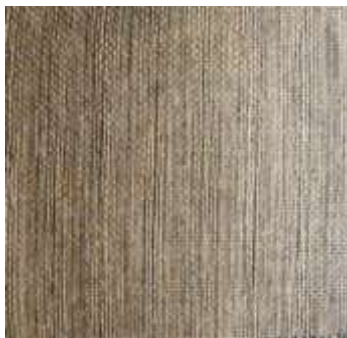
Jute woven fabric (Hessian cloth, 1×1 plain weave)
